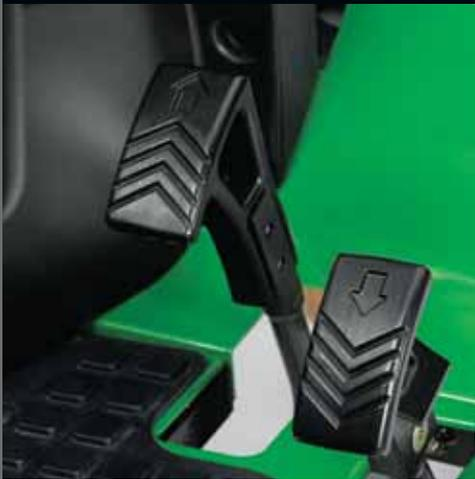
**Twin Touch™ transmission pedals** make it easy to switch from forward to reverse, and let you rest your heel on the platform the whole time you drive.
